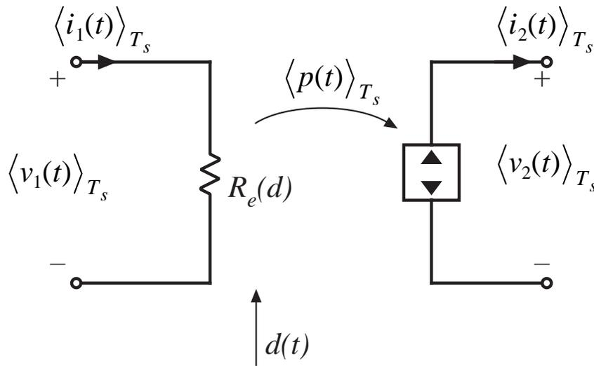
$$\langle i_1(t) \rangle_{T_s} = \frac{d_1^2(t) T_s}{2L} \langle v_1(t) \rangle_{T_s}$$
