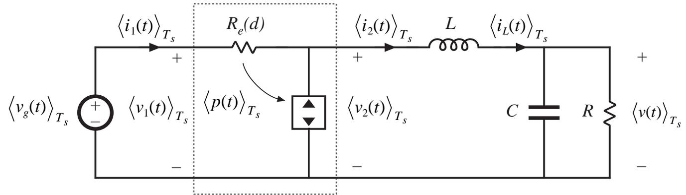
$$\mu(t) = \frac{\langle v_2(t) \rangle_{T_s}}{\langle v_1(t) \rangle_{T_s}} = \frac{\langle i_1(t) \rangle_{T_s}}{\langle i_2(t) \rangle_{T_s}}$$
