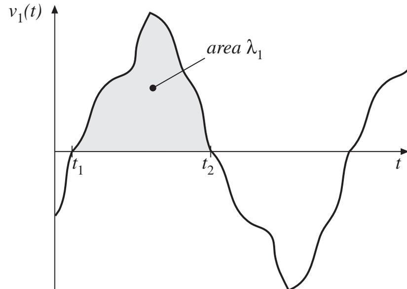
To attain a given flux density, the primary turns should be chosen according to
