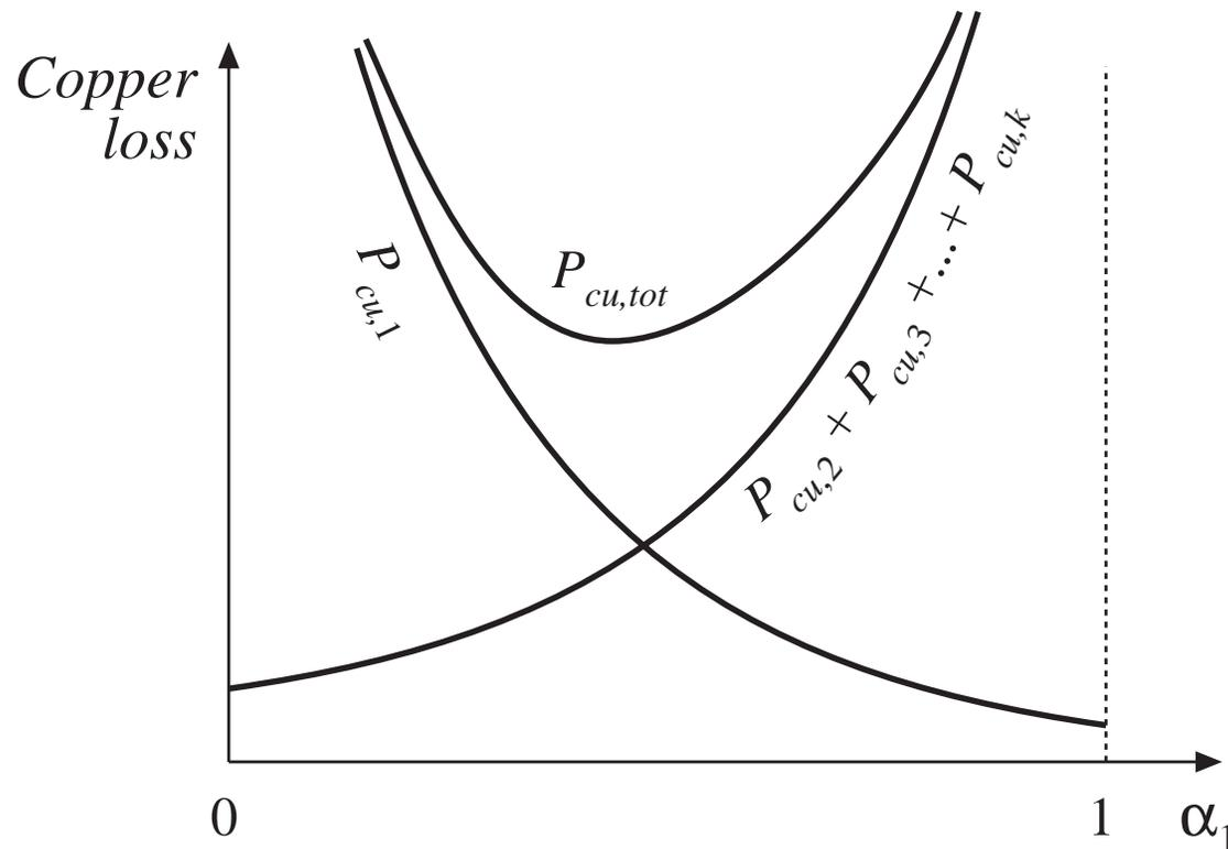
**For  $\alpha_1 = 0$ :** wire of winding 1 has zero area.  $P_{cu,1}$  tends to infinity
