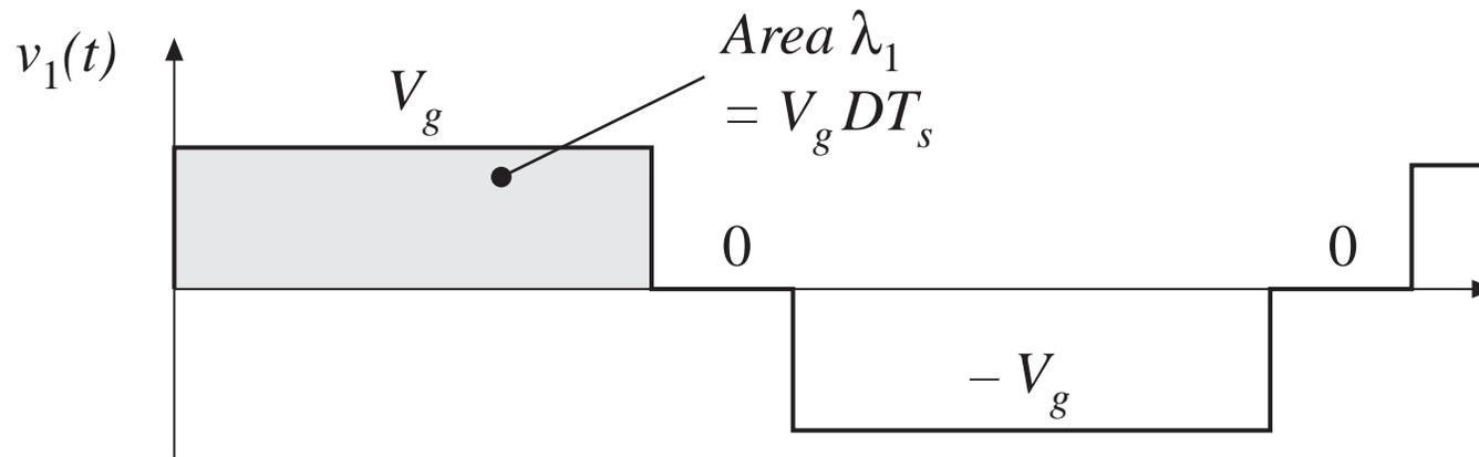
$$\lambda_1 = DT_s V_g = (0.75) (6.67 \mu\text{sec}) (160 \text{ V}) = 800 \text{ V}\text{-}\mu\text{sec}$$
