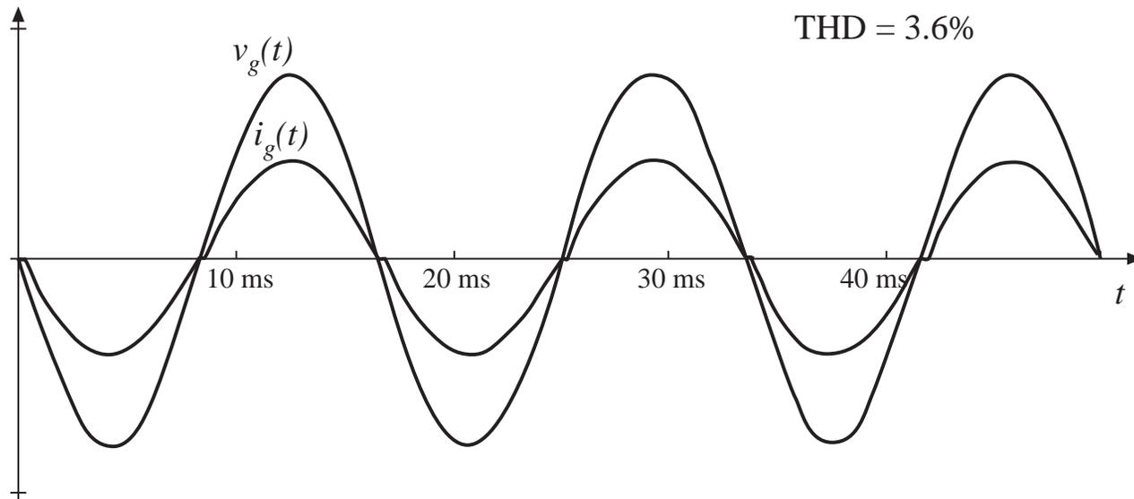
Typical ac line current and voltage waveforms, near the boundary between continuous and discontinuous modes and with small dc filter capacitor.  $f_0/f_L = 10$ ,  $Q = 1$
