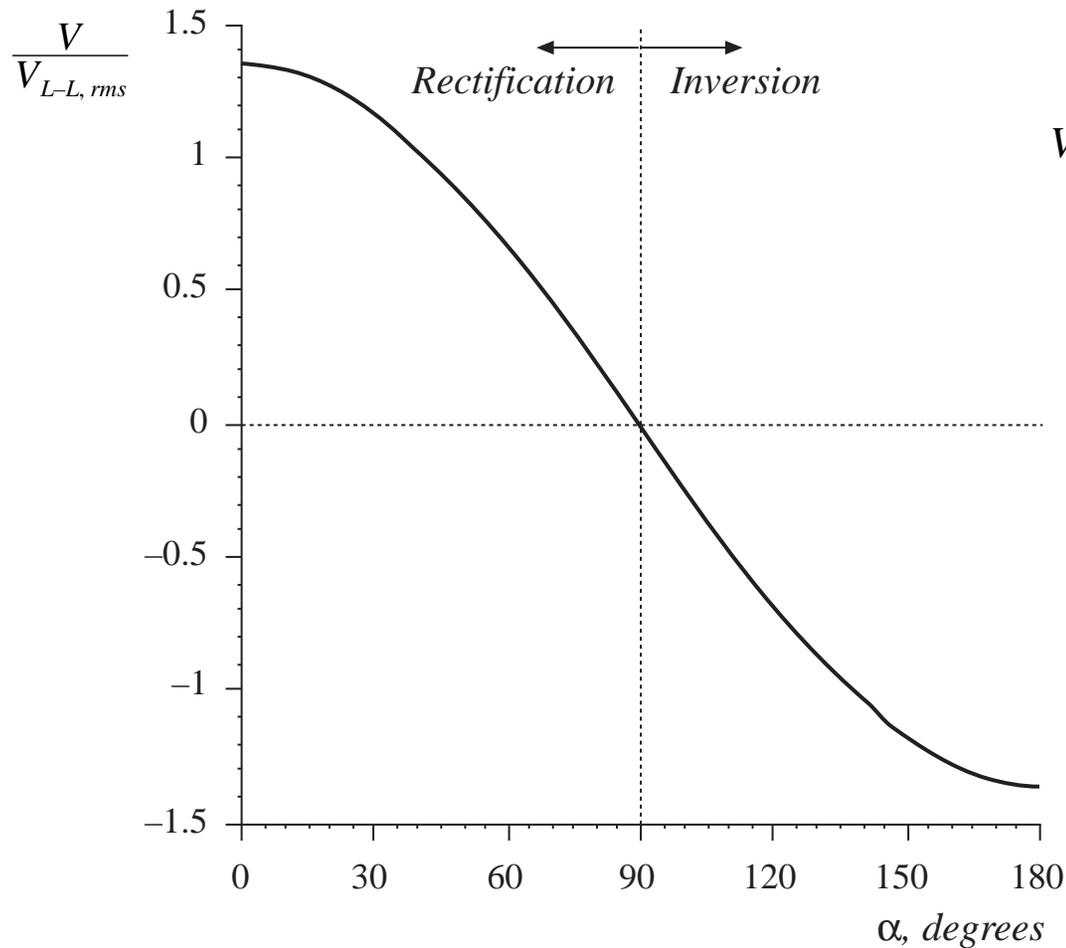
$$\begin{aligned} V &= \frac{3}{\pi} \int_{30^\circ+\alpha}^{90^\circ+\alpha} \sqrt{3} V_m \sin(\theta + 30^\circ) d\theta \\ &= \frac{3\sqrt{2}}{\pi} V_{L-L, rms} \cos \alpha \end{aligned}$$
