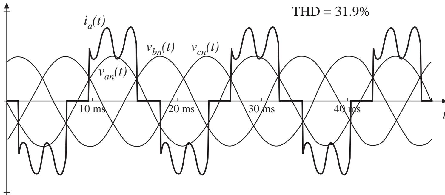
Inductor current contains sixth harmonic ripple (360 Hz for a 60 Hz ac system). This ripple is superimposed on the ac line current waveform, and influences the fifth and seventh harmonic content of  $i_a(t)$ .
