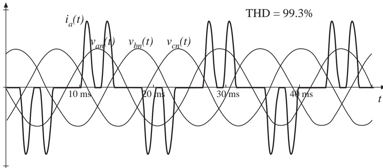
Phase  $a$  current contains pulses at the positive and negative peaks of the line-to-line voltages  $v_{ab}(t)$  and  $v_{ac}(t)$ . Distortion factor and THD are increased. Distortion factor of the typical waveform illustrated above is 71%.
