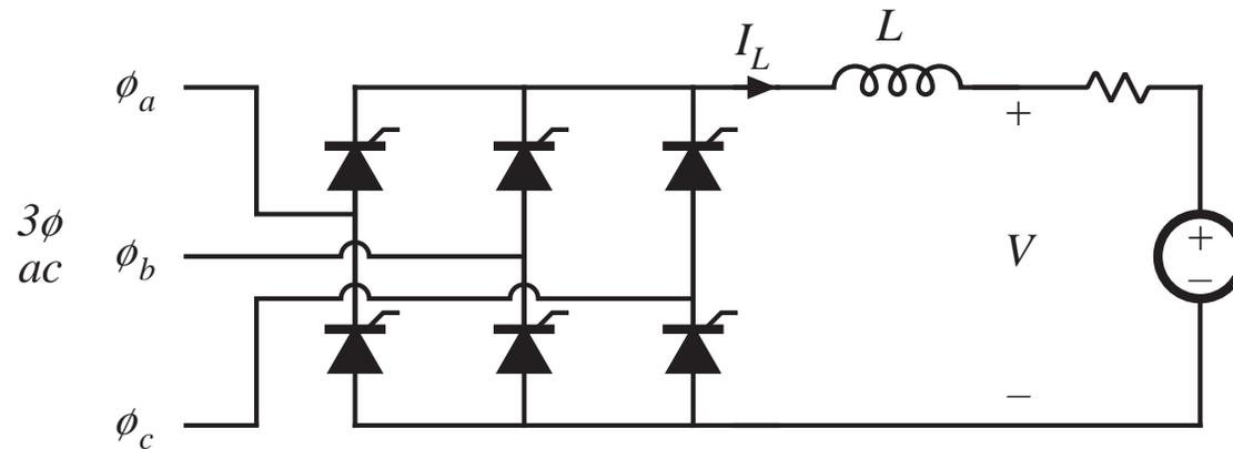
If the load is capable of supplying power, then the direction of power flow can be reversed by reversal of the dc output voltage  $V$ . The delay angle  $\alpha$  must be greater than  $90^\circ$ . The current direction is unchanged.
