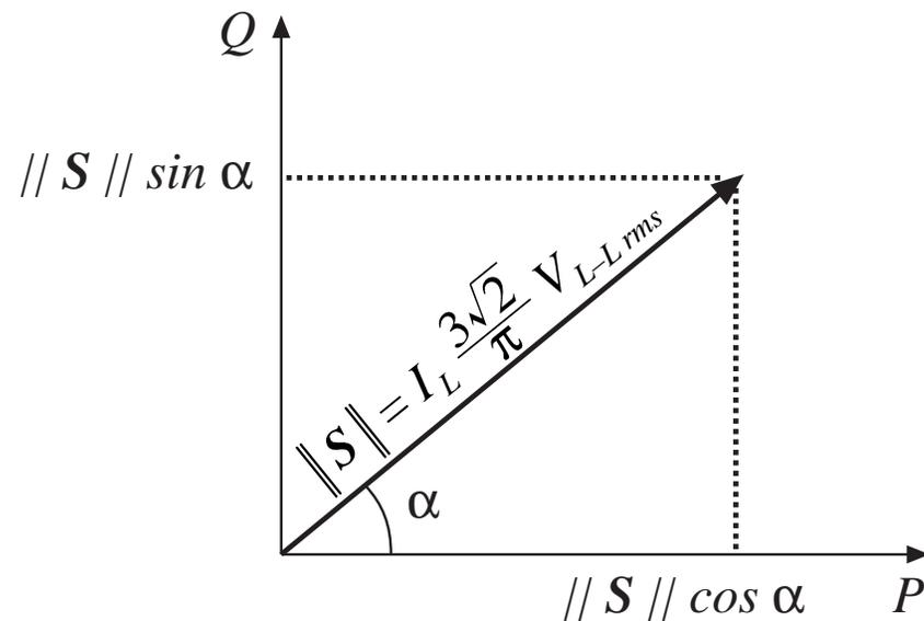
$$P = I_L \frac{3\sqrt{2}}{\pi} V_{L-L,rms} \cos \alpha$$
