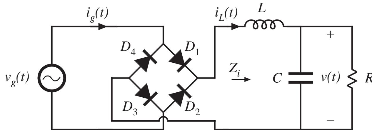
Full-wave rectifier with dc-side  $L$ - $C$  filter
