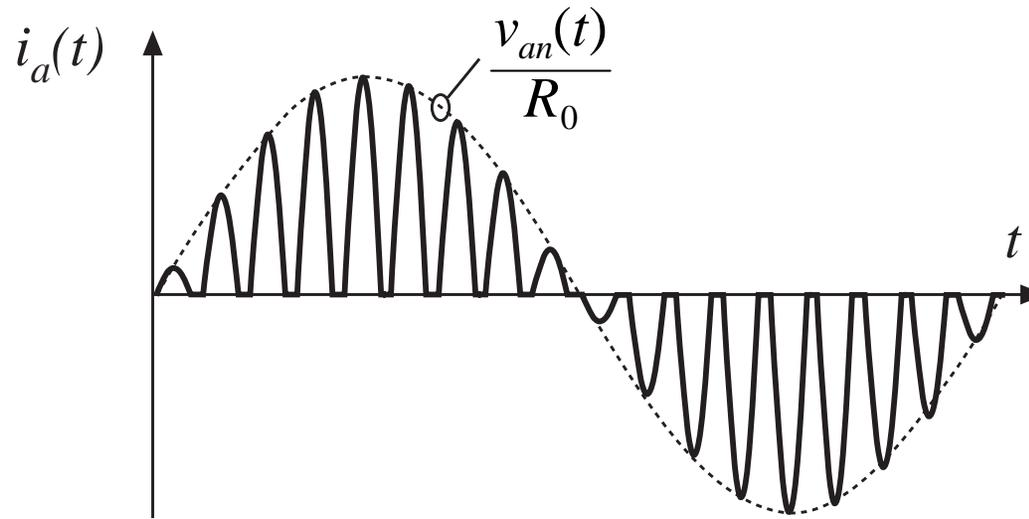
Input line currents are approximately sinusoidal pulses, whose amplitudes follow the input line-neutral voltages.
