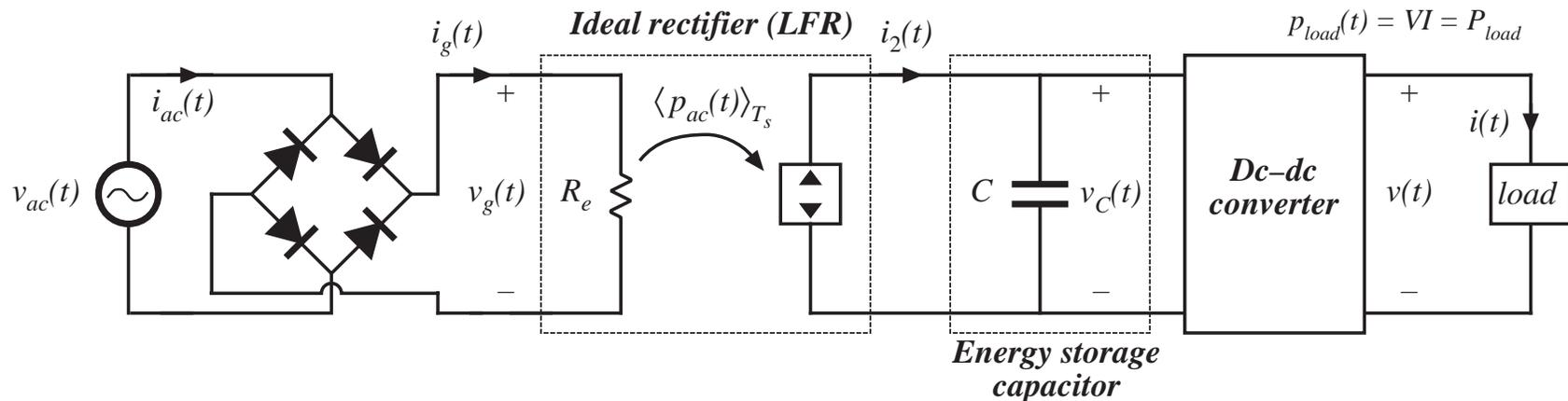
Energy storage capacitor voltage  $v_C(t)$  must be independent of input and output voltage waveforms, so that it can vary according to
