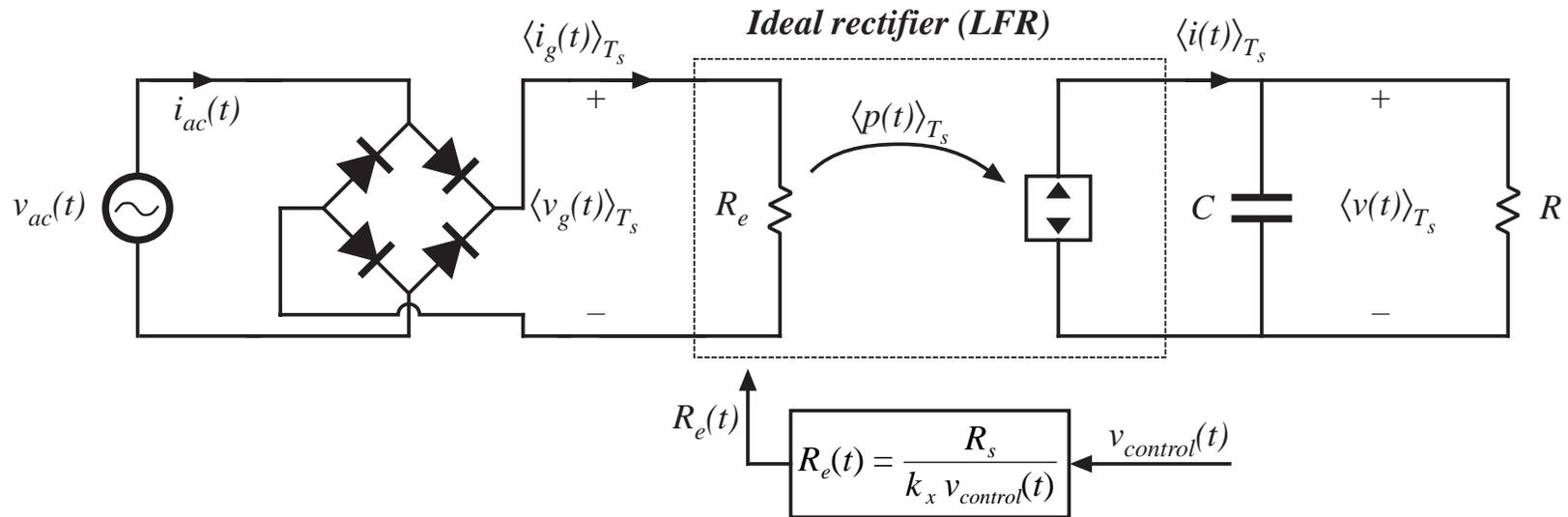
$$R_e(v_{control}(t)) = \frac{R_s}{k_x v_{control}(t)}$$
