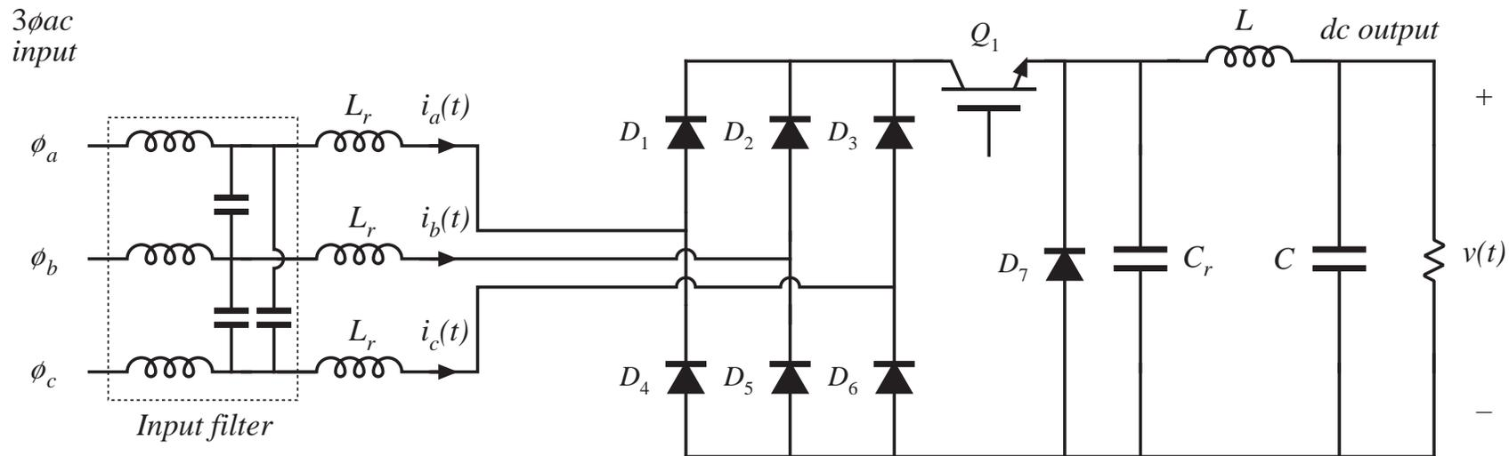
Inductors  $L_r$  and capacitor  $C_r$  form resonant tank circuits, having resonant frequency slightly greater than the switching frequency.
