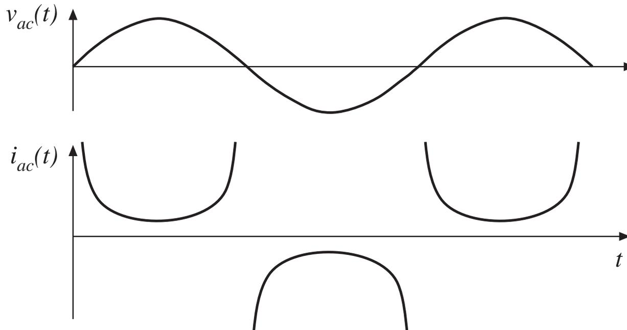
So bandwidth of capacitor voltage loop must be limited, and THD increases rapidly with increasing bandwidth
