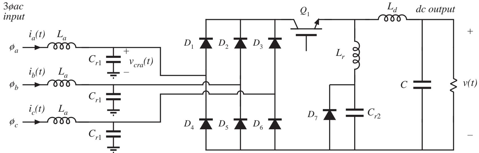
Inductors  $L_r$  and capacitors  $C_{r1}$  and  $C_{r2}$  form resonant tank circuits, having resonant frequency slightly greater than the switching frequency.
