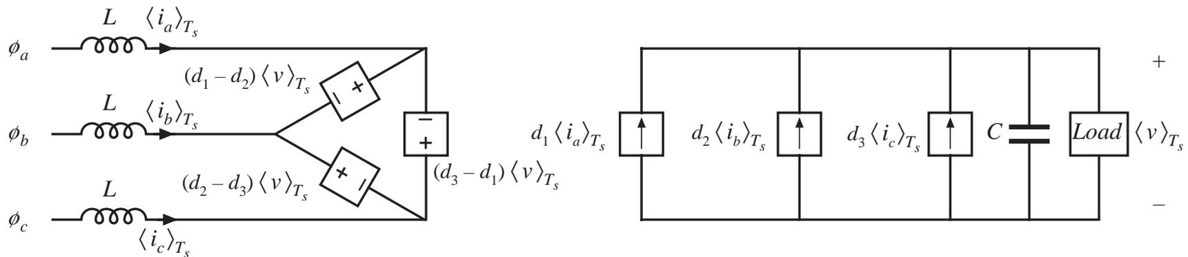
$$\langle v_{12}(t) \rangle_{T_s} = \langle v_{10}(t) \rangle_{T_s} - \langle v_{20}(t) \rangle_{T_s} = (d_1(t) - d_2(t)) \langle v(t) \rangle_{T_s}$$
