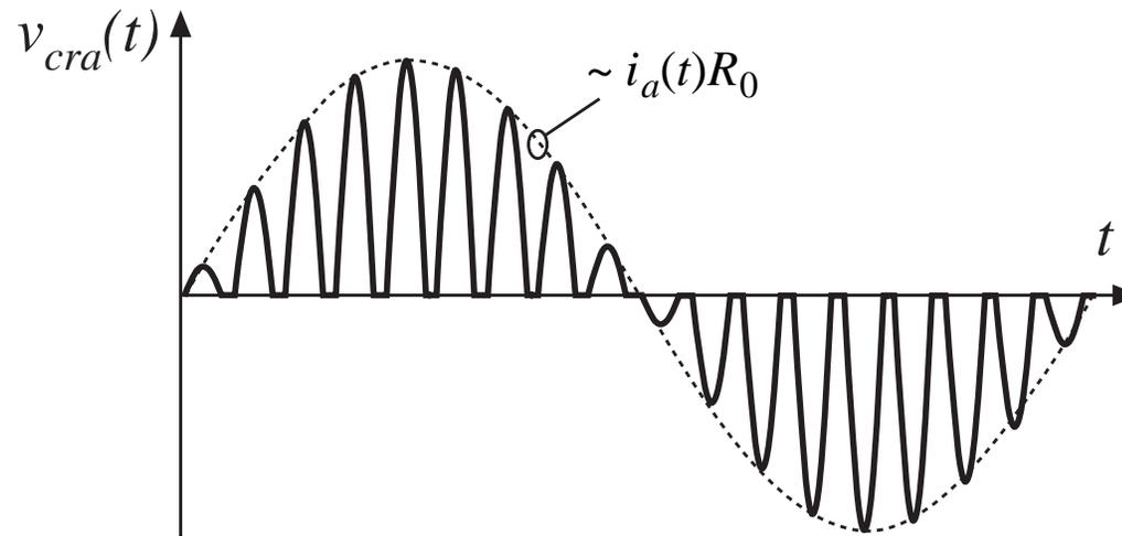
Input-side resonant voltages are approximately sinusoidal pulses, whose amplitudes follow the input currents. Input filter inductors operate in CCM.
