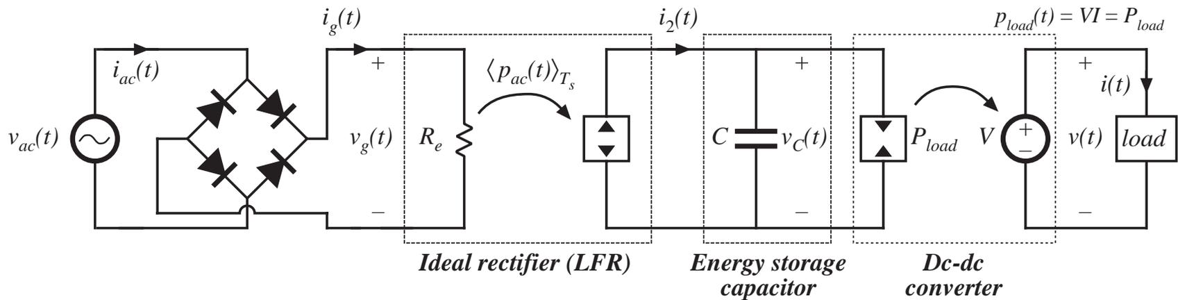
If the load power exceeds the average rectifier power, then there is a net discharge in capacitor energy and voltage over one ac line cycle.
