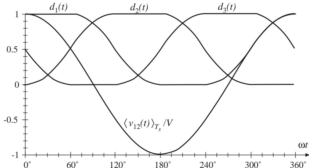
leads to undistorted line-line voltages provided that  $D_m \leq 1.15$ . The pulse width modulator saturates, but the duty ratio variations contain only triplen harmonics.  $V = V_{L,pk}$  is obtained at  $D_m = 1.15$ . Further increases in  $D_m$  cause distorted ac line waveforms.
