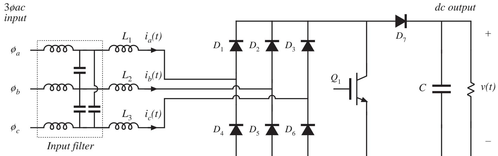
Inductors  $L_1$  to  $L_3$  operate in discontinuous conduction mode, in conjunction with diodes  $D_1$  to  $D_6$ . Average input currents  $\langle i_a(t) \rangle_{T_s}$ ,  $\langle i_b(t) \rangle_{T_s}$ , and  $\langle i_c(t) \rangle_{T_s}$  are approximately proportional to the instantaneous input line-neutral voltages. Transistor is operated with constant duty cycle; slow variation of the duty cycle allows control of output power.
