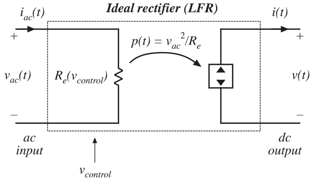
$$p(t) = \frac{v_{ac}^2(t)}{R_e(v_{control}(t))} \quad v(t)i(t) = p(t) = \frac{v_{ac}^2(t)}{R_e}$$
