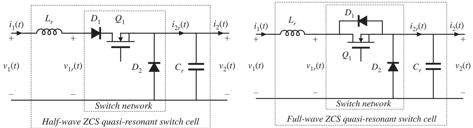
Insert either of the above switch cells into the buck converter, to obtain a ZCS quasi-resonant version of the buck converter.  $L_r$  and  $C_r$  are small in value, and their resonant frequency  $f_0$  is greater than the switching frequency  $f_s$ .
