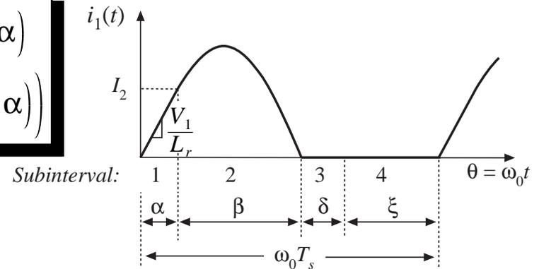
This subinterval ends at the first zero crossing of  $i_1(t)$ . Define  $\beta$  = angular length of subinterval 2. Then
