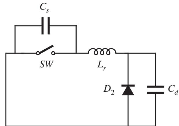
A half-wave version based on the PWM buck converter:
