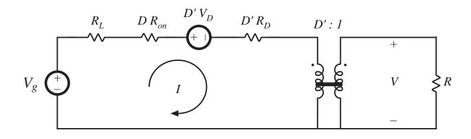
$$V = \left(\frac{1}{D'}\right) \left(V_g - D'V_D\right) \left(\frac{D'^2R}{D'^2R + R_L + DR_{on} + D'R_D}\right)$$
