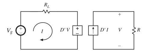
The dependent sources are equivalent to a D': I transformer:
