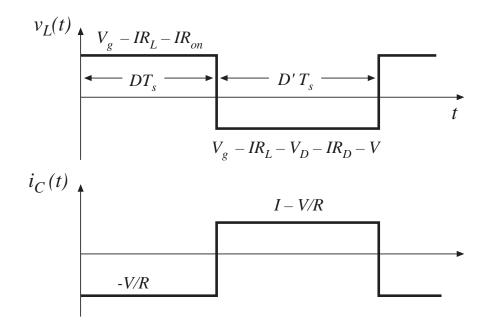
$$\langle v_L \rangle = D(V_g - IR_L - IR_{on}) + D'(V_g - IR_L - V_D - IR_D - V) = 0$$
