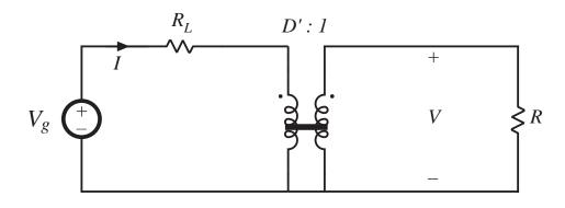
$$I = \frac{V_g}{D'^2 R + R_L} = \frac{V_g}{D'^2} \frac{1}{1 + \frac{R_L}{D'^2 R}}$$
