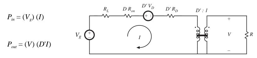
$$\eta = D' \frac{V}{V_g} = \frac{\left(1 - \frac{D'V_D}{V_g}\right)}{\left(1 + \frac{R_L + DR_{on} + D'R_D}{D'^2R}\right)}$$
