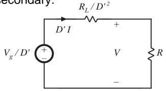
Solution for output voltage using voltage divider formula:
