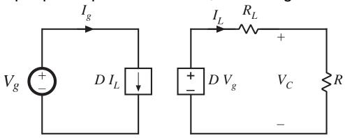
Replace dependent sources with equivalent dc transformer:
