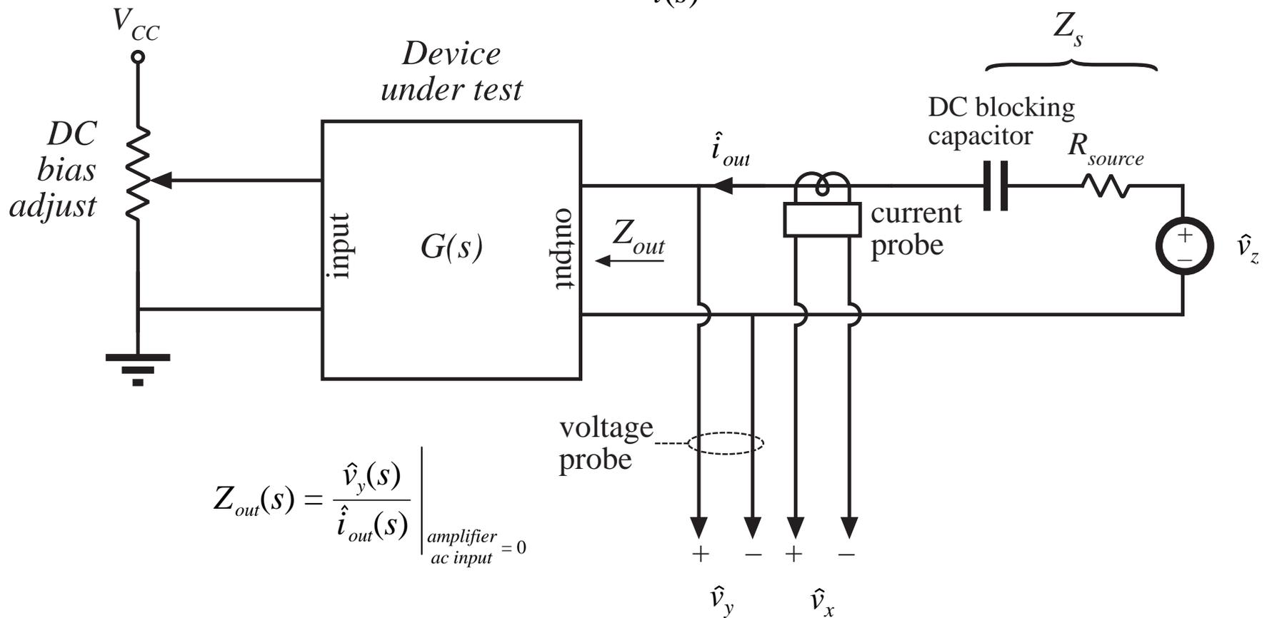
$$Z_{out}(s) = \frac{\hat{v}_y(s)}{\hat{i}_{out}(s)} \Bigg|_{\substack{\text{amplifier} \\ \text{ac input} = 0}}$$
