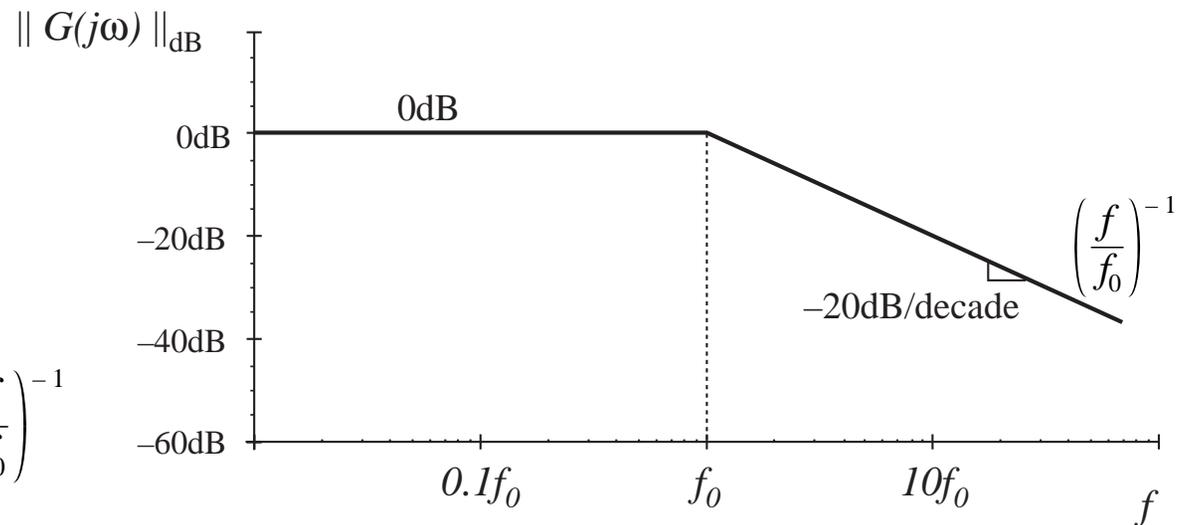
The high-frequency asymptote of  $\|G(j\omega)\|$  varies as  $f^{-1}$ . Hence,  $n = -1$ , and a straight-line asymptote having a slope of -20dB/decade is obtained. The asymptote has a value of 1 at  $f = f_0$ .
