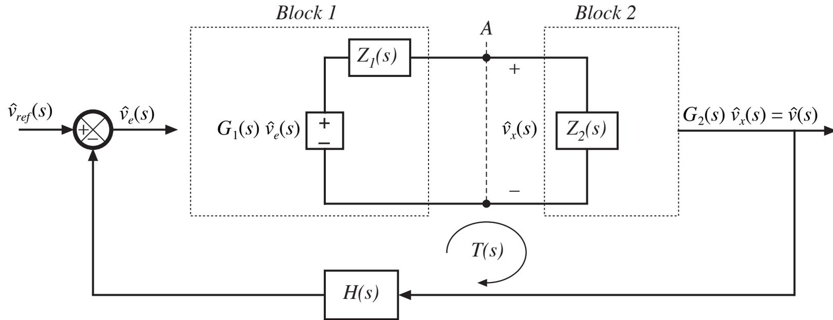
Objective: experimentally determine loop gain  $T(s)$ , by making measurements at point A
