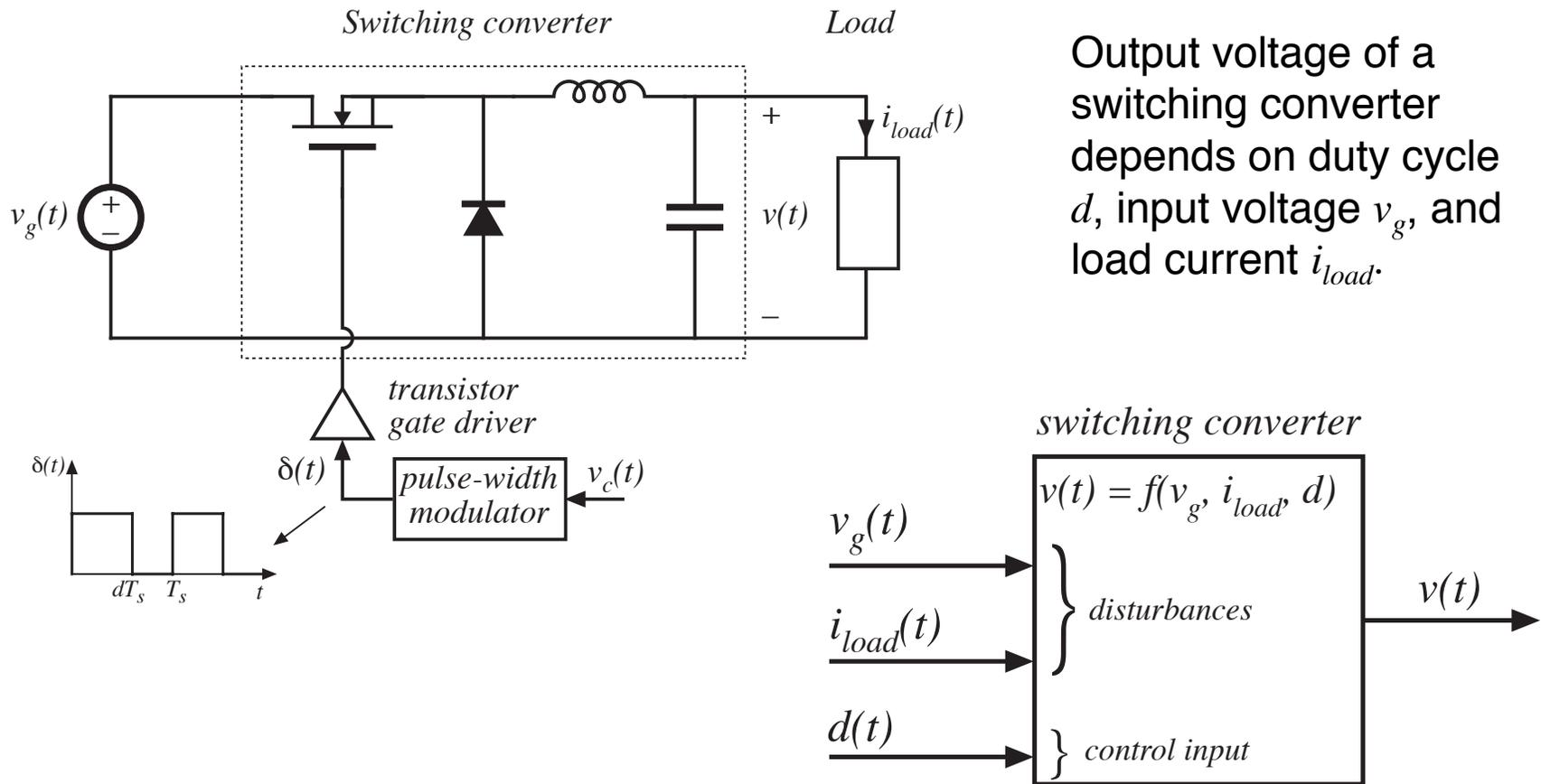
Output voltage of a switching converter depends on duty cycle  $d$ , input voltage  $v_g$ , and load current  $i_{load}$ .
