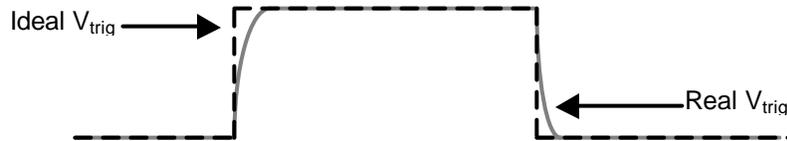
**Figure 2.12** Ideal and Real Waveforms of Control Signal
